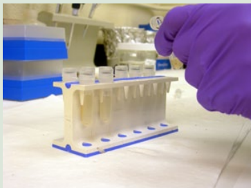
3. DNA is extracted and placed in small tubes with small beads coated with a matching DNA probe that selects for A. vitis DNA and leaves behind DNA from the plant and other microorganisms that could interfere with the test.
